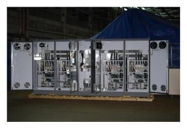
• Regenerative Inverter for Dynamometer. Example 20 HP. Customer: Magtrol
