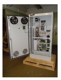
• Ventilation Fan Inverters for the gold mining industry. Example: 150 HP, 350 HP Customer: Epitron, Inc.
