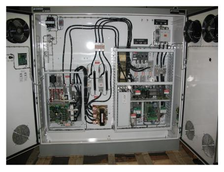
• Draw Works and Mud pump Inverters for the oil industry. Example: 1200 HP Regenerative Draw Works Inverter and 1000 HP Mud Pump Inverter with input power supplied by diesel generators. Customers: Stewart & Stevenson, Estrella Servicios Petroleros S.A.
